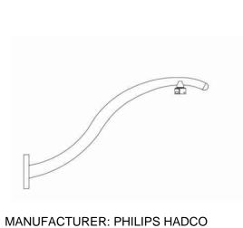
URBAN LUMINARE: WESTBROOK CXF14 POLE: 13' DECORATIVE CAST ALUMINUM ARM: SINGLE (HFP710) FOOTING: AB CHANCE - C11242NG4TK W/ROUND MOUNTING PLATE FINISH: BLACK DARK SKY FRIENDLY 17400 SW UPPER BOONES PROVIDE AUTO PROFILE DIMMING - COORDINATE PROFILE WITH CITY OF WILSONVILLE AND MANUFACTURE
