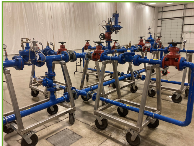
Control valve training demonstration setup
