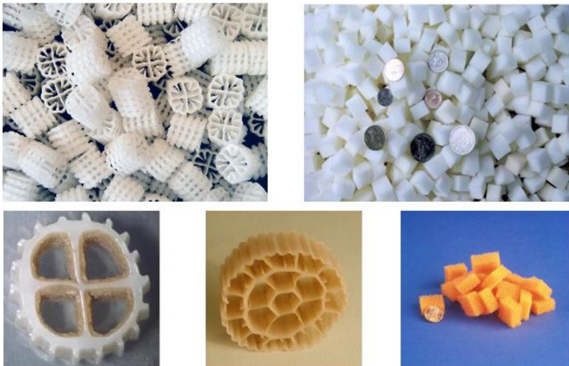
Figure 6.5 Examples of “Wagon Wheel” and Sponge Media Used in an IFAS Technology
