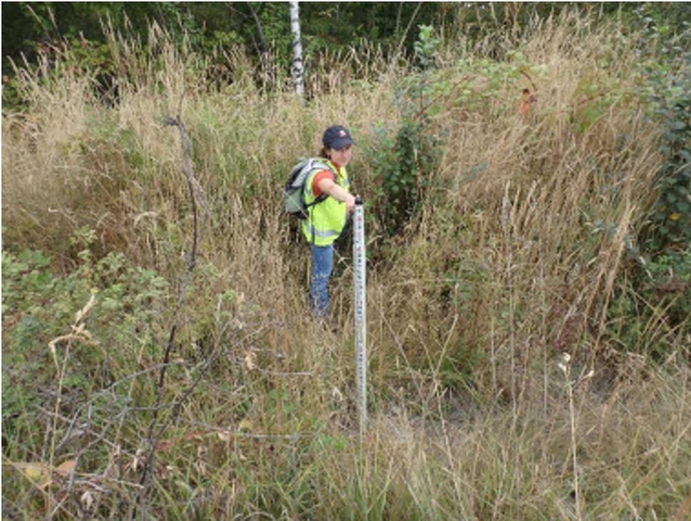
Figure 4. East ditch vegetated with grasses and left bank at 2.5 foot height. (node 6)
