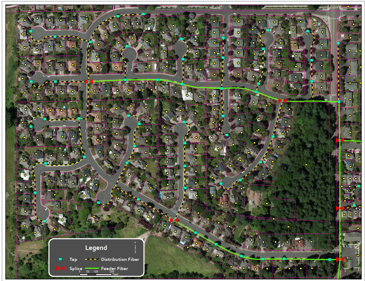
Figure 20: Sample FTTP Access Layer Design
