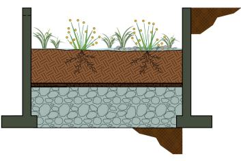
Infiltration planters installed adjacent to building footage and foundations should be installed with a waterproof liner between the facility and building.
