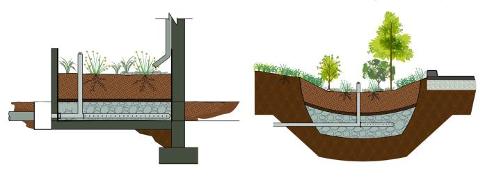
Example cross section for filtration stormwater planter
