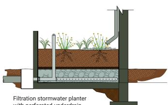
Filtration stormwater planter with perforated underdrain, liner, and overflow.
