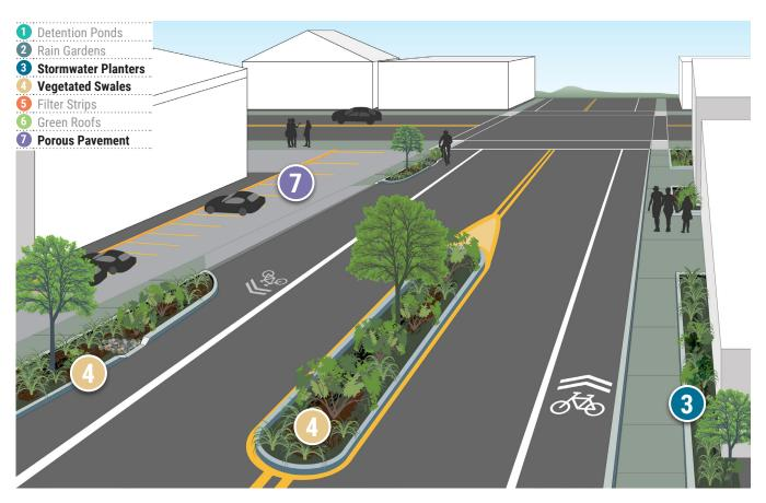
Example of stormwater management facilities applied to a transportation corridor. Applicable facilities are highlighted, as not all types of facilities may be used at a site. Source: Brown and Caldwell
