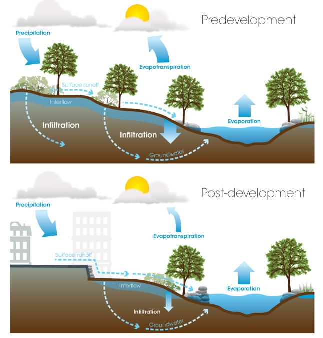
Impervious areas associated with development reduce interflow and infiltration, resulting in an increased rate, volume, and duration of overland flows. Source: Brown and Caldwell
