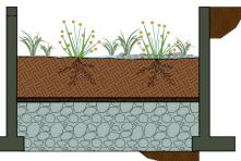
Infiltration stormwater planter is unlined to promote infiltration.
