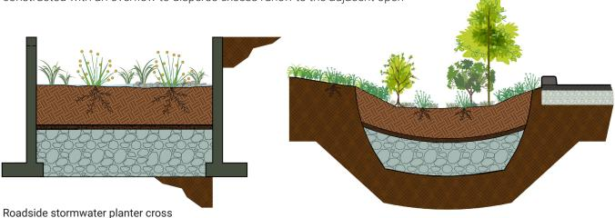
Roadside stormwater planter cros section example.
