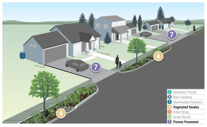
Examples of stormwater facilities used in a residential development. Applicable facilities are highlighted, as not all types of facilities may be used at a site. Source: Brown and Caldwell
