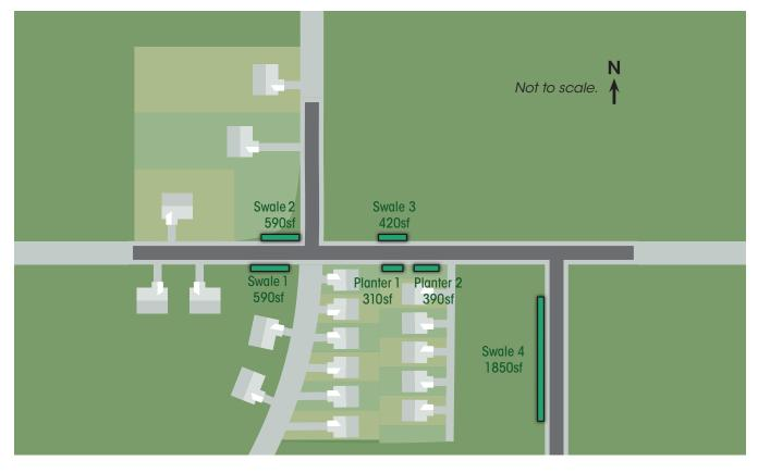
Example site layout schematic with offsite drainage areas defined.
