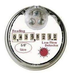
**Reading:** (meters 1" or smaller) The reading starts on the 4<sup>th</sup> place from the left hand side. Ignore the commas and decimal. The sample above reads 439.
