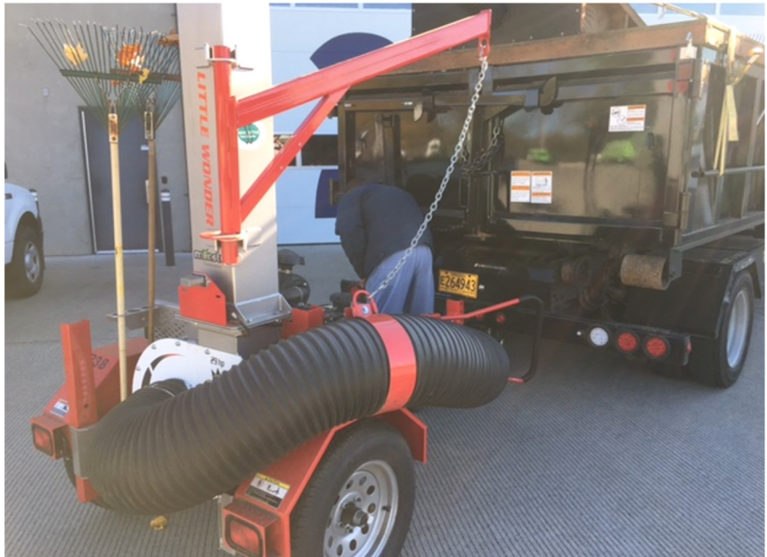
Fleet Mechanic Scott Wright repairs wiring on a leaf vacuum unit
