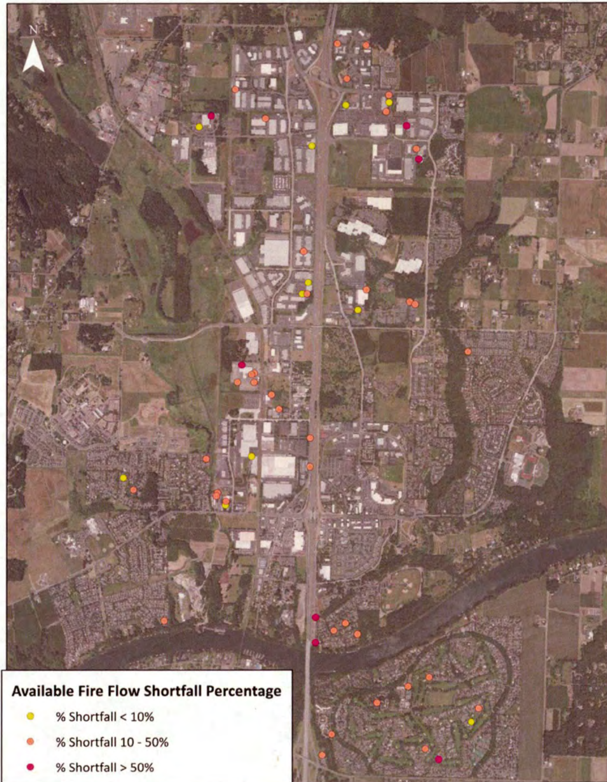
CHART 3.1 – Wilsonville Localized Fire Flow Deficiencies
