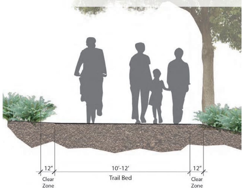
Figure 31. Boeckman Creek Regional Trail Cross-Section
