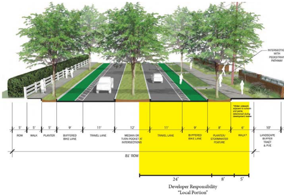
Figure 3. Boeckman Road, including developer responsibility/local portion
