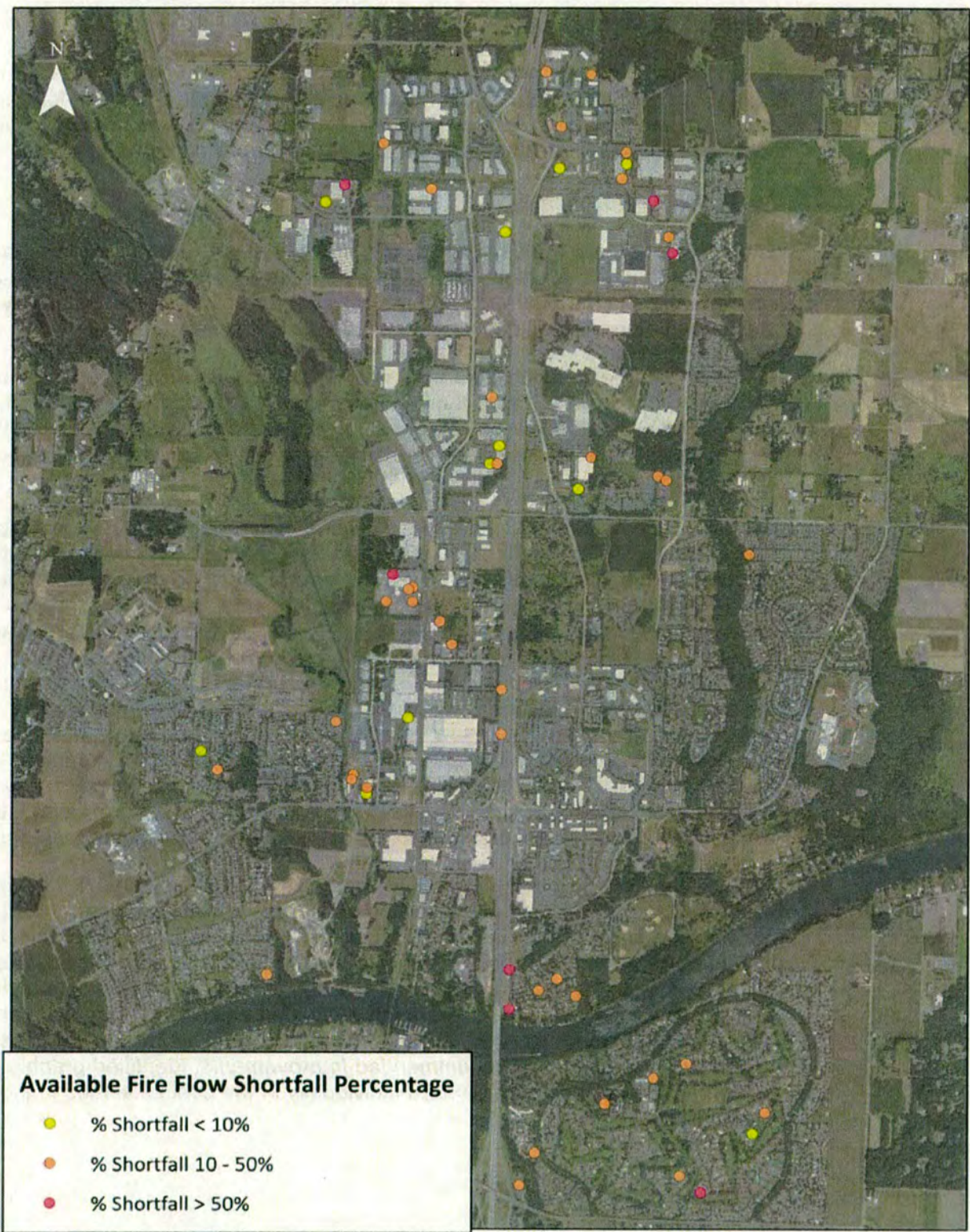
CHART 3.1 - Wilsonville Localized Fire Flow Deficiencies
