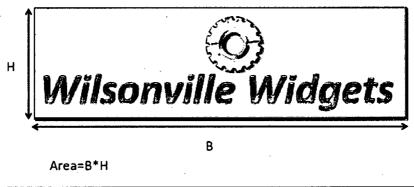
Figure 1. Measurement of Cabinet or Similar Signs
